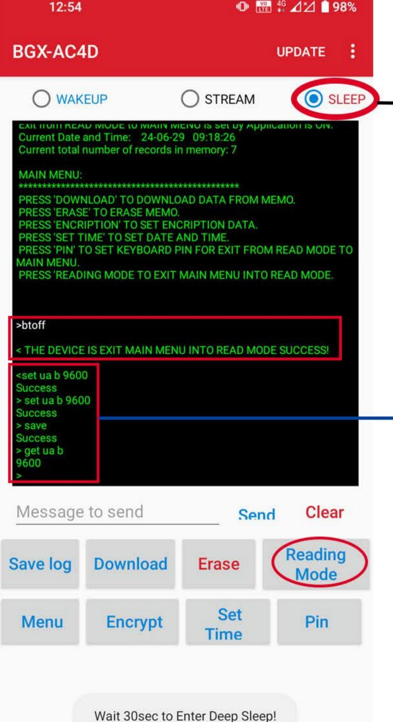
When this message appears "set ua b 9600" Success it means device has entered Deep Sleep successfully to access menu again you must WAKEUP device when entering menu after each manipulation, you MUST reenter SLEEP mode again You must wait 30 seconds before device goes into Reading mode after closing app, if using "PIN" Fonction this sleep mode is not necessary since Bluetooth is completely off in this mode. Sleep fonction is only to reduce Bluetooth Always On fonction.
